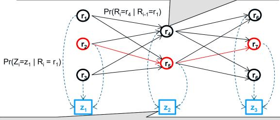
observable variable  $Z = (Z_1, ..., Z_n) \rightarrow$  position measurements (e.g. GPS)
